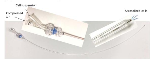
Figure 1: Microjet<sup>™</sup> Sprayer optimized for high cell viability and access in decellularized lungs
